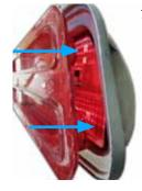
1. Slide the lens/LED assembly into the housing.
