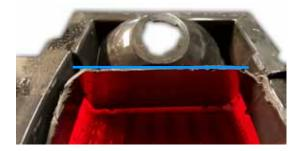
7. Cut away the remaining triangular plastic areas so that the light emitted from the LED panel will not be blocked. Also make sure that the cut away area does not stick up over the housing ledge.
