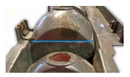
5. First cut around the upper bucket. Break it away from the housing then continue to the lower section.
