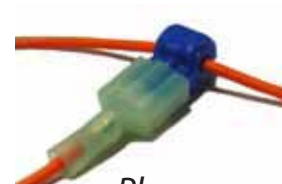
Plug connector into T-Tap
