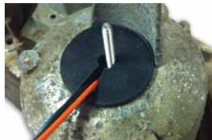
Use the end of the screw to adjust the LED panel into its final position. Place the slotted washer on top of the grommet. Then slide on the nylon washer and screw it all together with the black wing nut. Tighten snug until the LED panel is fit snug in place. Make sure that the LED panel is not bending in from too much tightening force. You may want to use loctite or silicone to make sure the wing nut stays secure.
