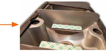
Now move down to the brake light pocket. Locate the upper edge (closest to the center pocket). Measure from the edge down 3/4" and mark. Peal off the protective strip and attach a mounting bracket so that the edge of the bracket lines up with the mark.
