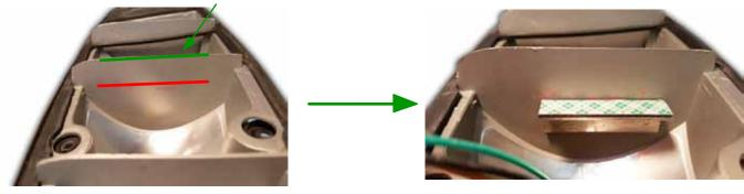
4. Locate the lower edge (opposite of the center pocket). Measure from the edge down 3/4" and mark. Peal off the protective strip and attach a mounting bracket so that the edge of the bracket lines up with the mark.
