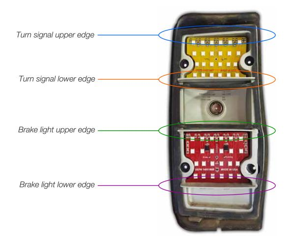
Locate the upper edge (opposite of the center pocket). Measure from the edge down 3/8" and mark. Peal off the protective strip and attach a mounting bracket so that the edge of the bracket lines up with the mark.
