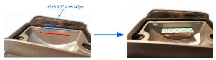
Locate the lower edge (closest to the center pocket) Measure from the edge down 1" and mark.
