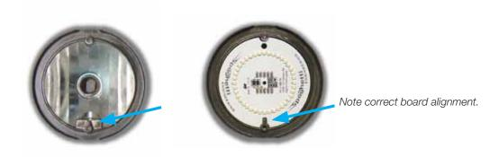
2. Reinstall the gasket and lens onto the housing. Align the lens into position and carefully screw down. Make sure the LED board is sitting flush. The Lens will hold the LED board into place. Be careful not to over tighten the lens.
