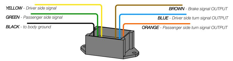
The DIGI-TAILS Taillight Signal Separator will convert the Passenger and Driver signals with no dedicated brake light signal and output a driver side turn signal, passenger side turn signal, and Brake light
