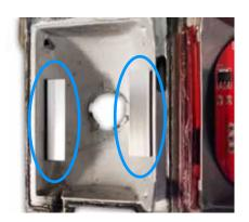
**4.** For the other 3 pockets, mount the brackets on the horizontal ends. Again, measure down 5/8" from the edge and attach the brackets.
