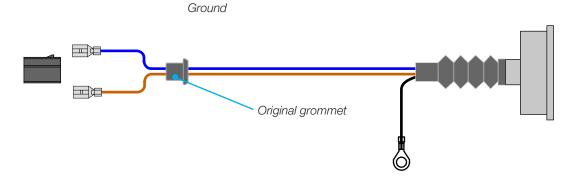
Attach the female blade terminals onto the LIGHT BLUE, DARK BLUE, and BROWN wires. Attach the ring terminal onto the BLACK wire and connect to a good ground. Crimping the terminals is satisfactory, however, soldering the connection is preferred. Insert the female blade terminals into the connector as shown.
