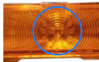
Circle of LEDs on LED panel matches center circle of lens.
