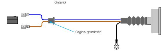
Attach the female blade terminals onto the **LIGHT BLUE**, **DARK BLUE**, and **BROWN** wires. Attach the ring terminal onto the **BLACK** wire and connect to a good ground. Crimping the terminals is satisfactory, however, soldering the connection is preferred. Insert the female blade terminals into the connector as shown.
